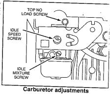
DO NOT ADJUST TOP SPEED SCREW. It is pre-set at factory.
