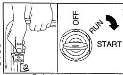
Use short starting cycles (15 secs. per min.) to prolong starter life. Extended cranking can damage starter motor.
