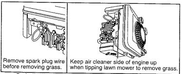
Periodically remove grass build-up under mower deck
