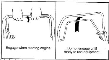
Typical safety brake control handle Typical traction control handle
